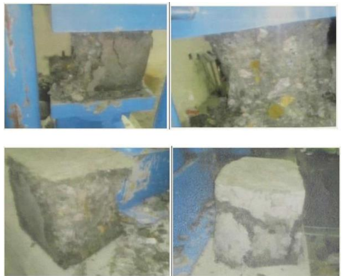
Fig 5: Specimens after compression testing.
