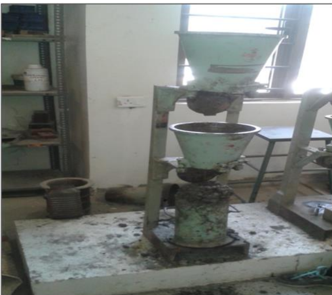
Compaction factor test
