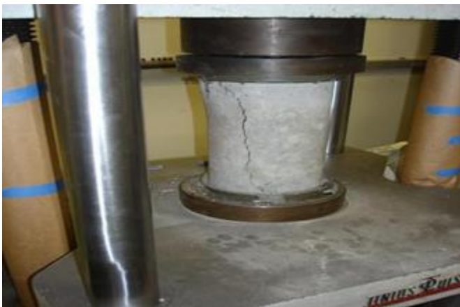
Fig 2: compressive strength test
