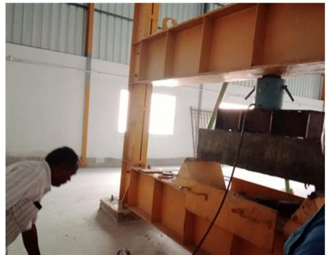
Testing of RCC beam
