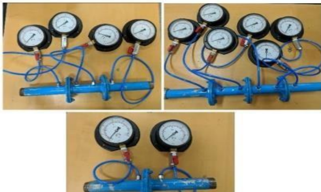
Fig. 3: Pressure gauge arrangements for 1-stage, 2-stage & 3-stage assembly
