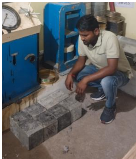
Fig 5.5: Cubes Casting and setting
