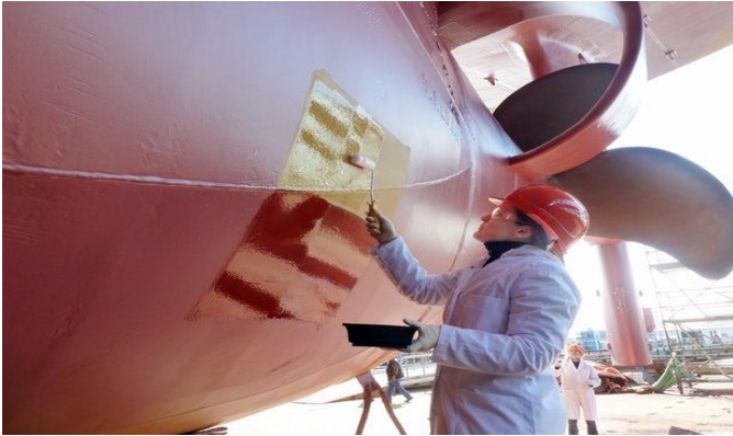
Figure 12. An engineer applying coating to a ship's hull
