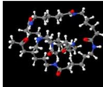
Fig-3: Molecular structure of Nylon 6.6
