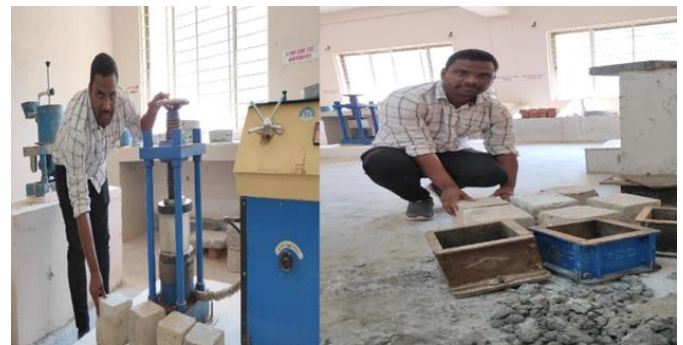
Fig 1 Apparatus for Compressive Strength Test
