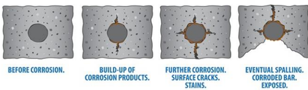
FIGURE 1. CORROSION OF REINFORCED CONCRETE OVER TIME [16]
