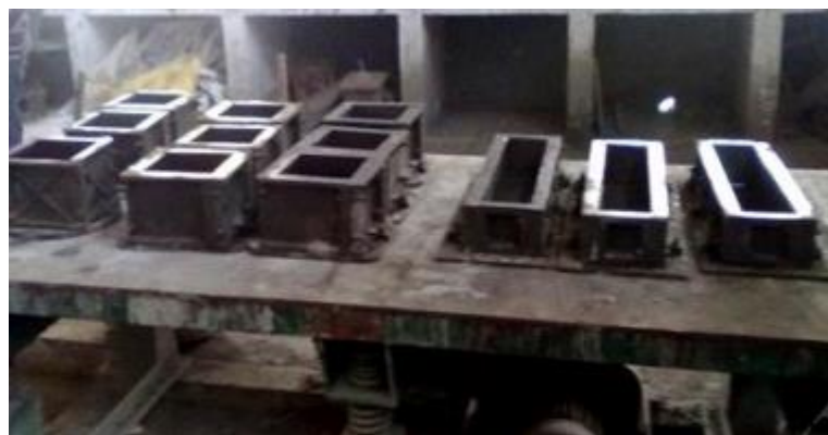
Fig 2 Steel cubes and moulds used in current experimental work
