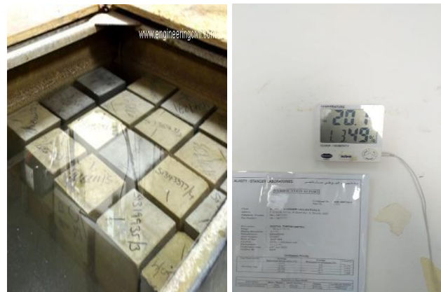
Cube submerged in curing tank
