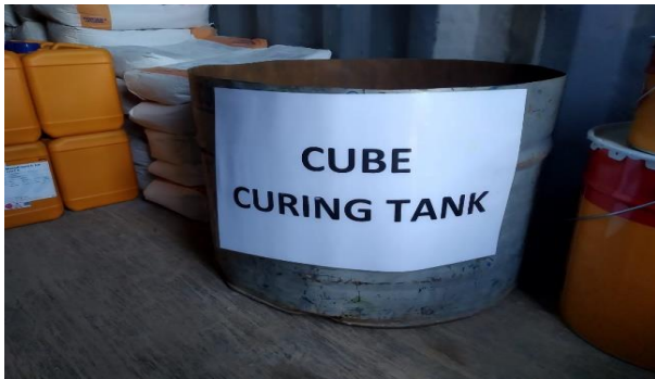
Temporary Cube tank
