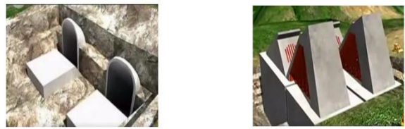
Fig-1: Construction of concrete anchorage
