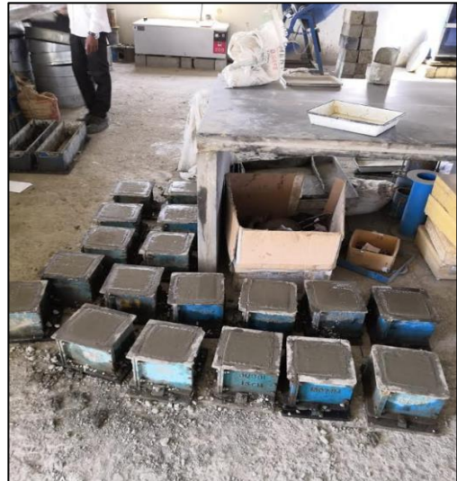
Figure 2 Casting of Cubes and Beams
