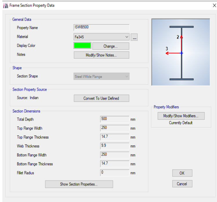
Fig 6 Defining Column Section
