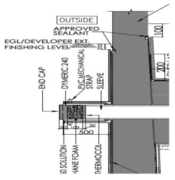
Advatages : Necessisity of breaking the block works during service cable entry not required. Water proofing not damaged. Chances of water penetration inside basement is zero.
