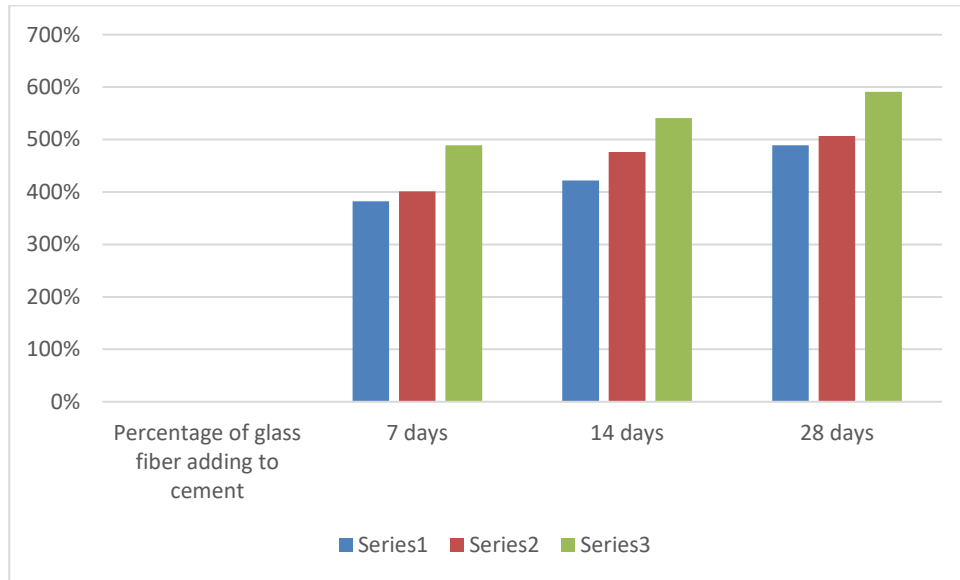
Fig 2 Glass fibers and Bacillus megaterium MTCC 105 cells/ml and 5 grams of calcium lactate vs flexural strength
