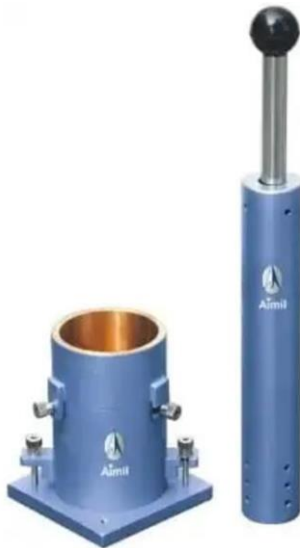
Figure 6. Apparatus for Proctor's Compaction Test
