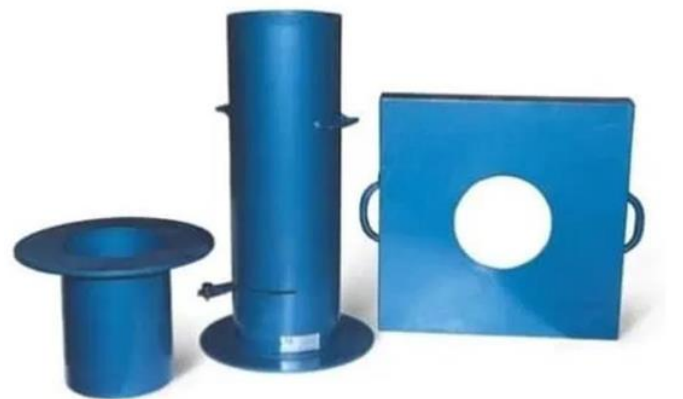
Figure 4. Apparatus for Sand Replacement method Test
