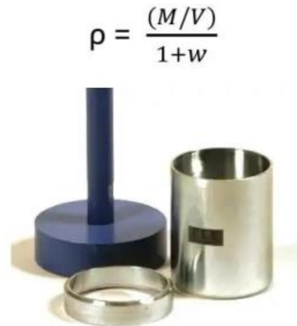
Figure 3. Apparatus and Formula for Core Cutting Method
