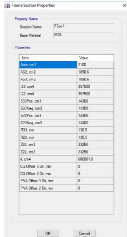
Fig 4 (b) Defining Frame Section Properties
