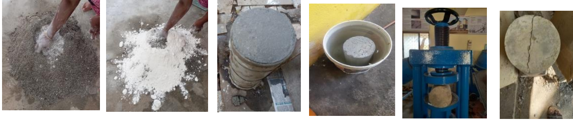
Fig.7 – Casting and Testing of Split Tensile Strength of Cylinder
