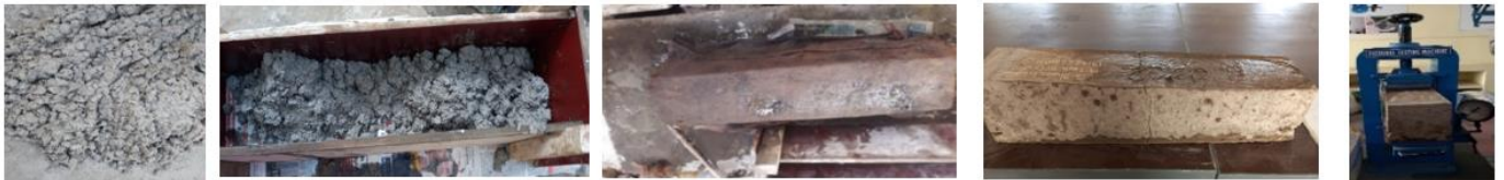
Fig.9 – Casting and Testing of Flexural Strength of Be
