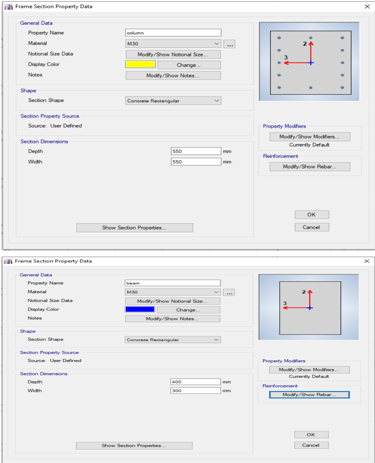
Fig 14: Defining section properties of beam and column.
