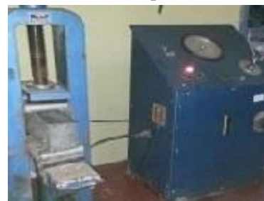
(c) Flexural strength test
