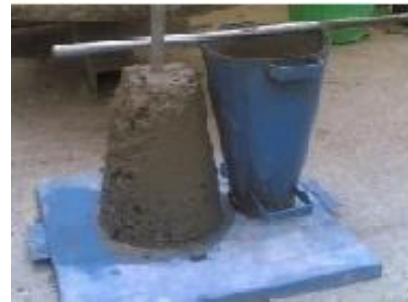
(b) Slump test
