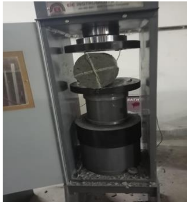
Fig:- Split Tensile Strength Test
