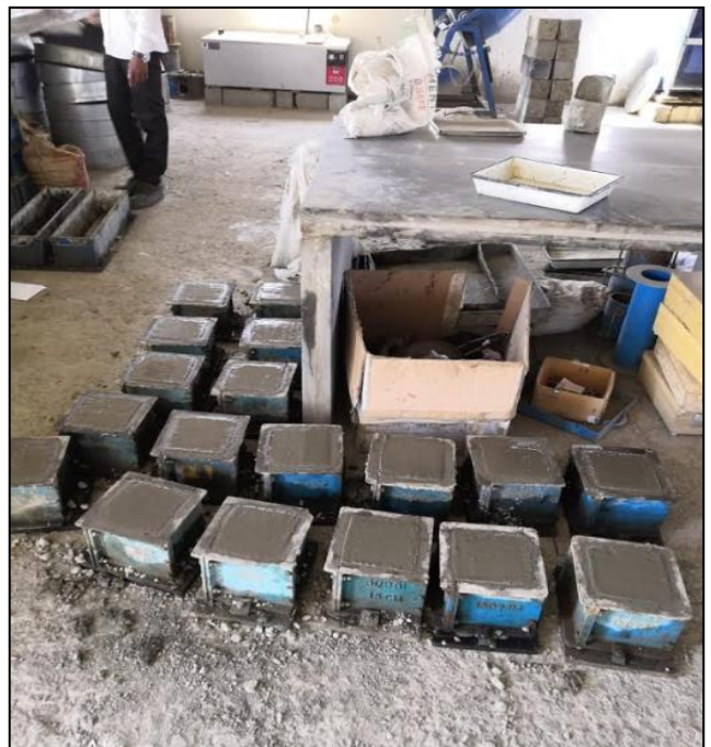
Figure 3 Casting of Cubes and Beams
