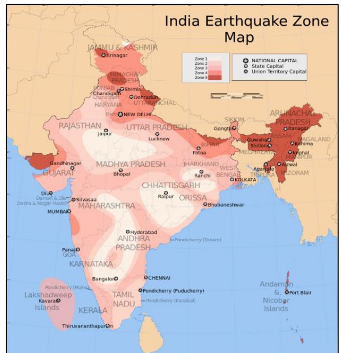
Fig 2: Seismic regions as per I.S. 1893-I:2016
