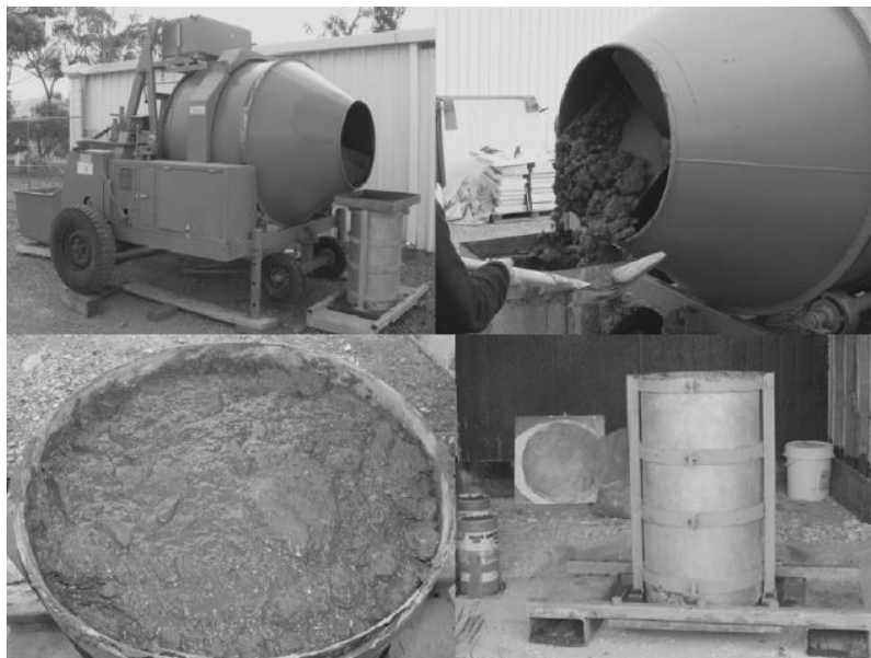
Figure 4 .Sample mixing and casting
