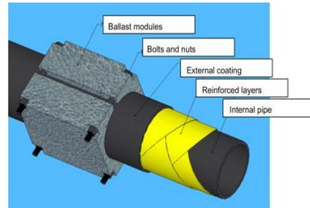
**Fig-4: Gravity anchor**
