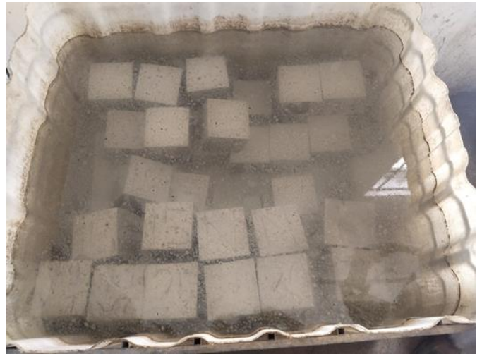
Figure 6 : Curing of Cube
