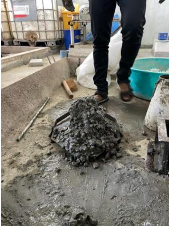
Figure 3: Slump Cone Experiment
