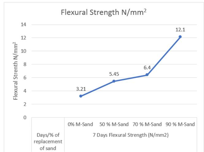
Fig 5 : Flexural Strength
