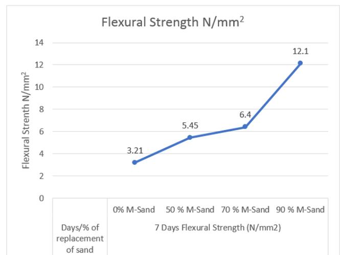
Fig 5 : Flexural Strength
