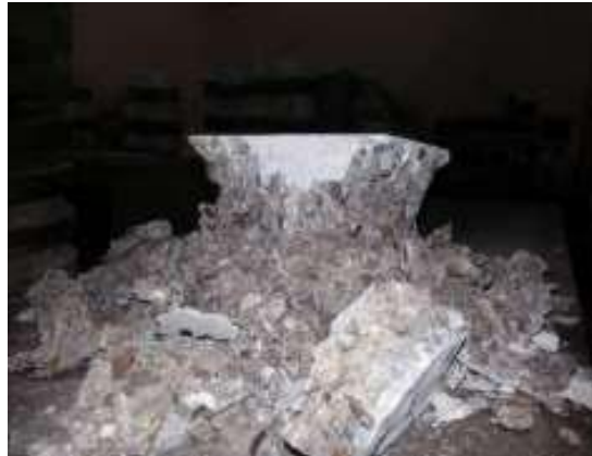
Plate 2. Test of compressive strength of concrete
