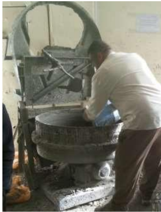
Plate 1. Rotary concrete mix used in this study
