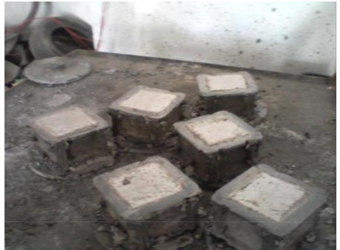
Figure 5. Casting of geo-polymer concrete cube
