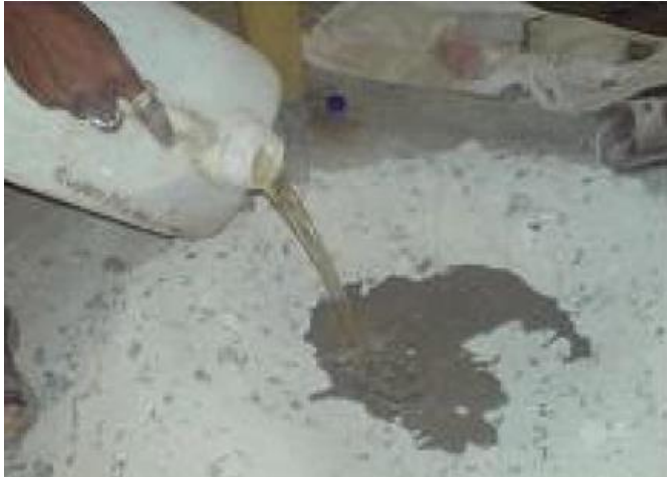
Figure 3. Adding sodium silicate solution to dry mix
