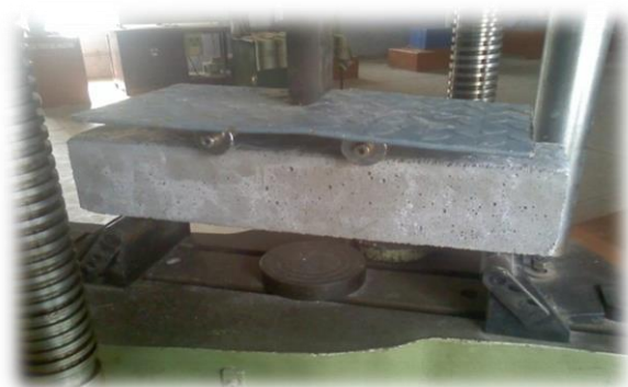
Figure 6. Flexural Strength Test on Specimens
