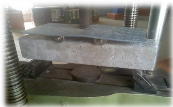
Figure 6. Flexural Strength Test on Specimens
