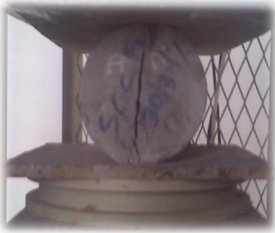
Figure 7. Split Tensile Strength Test on Specimens
