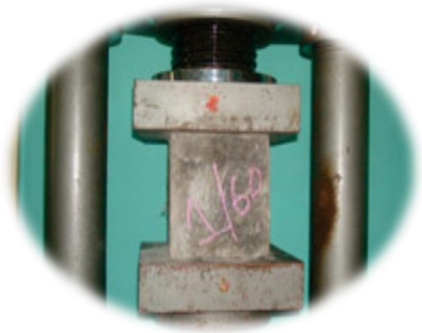
Figure 5. Compression Test on Specimens
